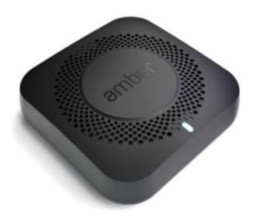
The device is not large, being 4.75" square by 1.25" thick and is fairly light.
