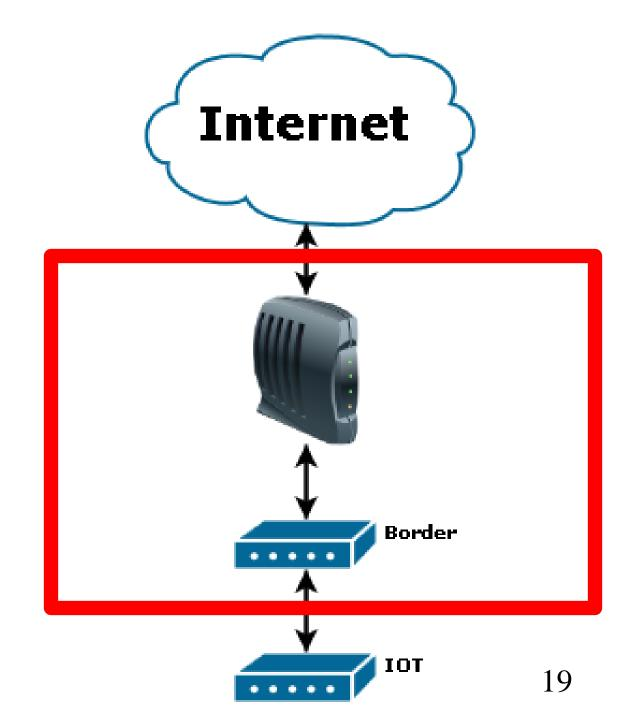
Therefore, for most of us, adding one additional router brings us to the "two router" configuration:
