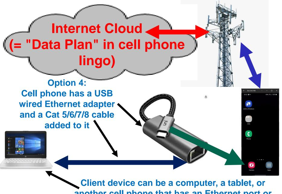
Client device can be a computer, a tablet, or another cell phone that has an Ethernet port or adapter 6
