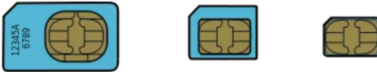
From left to right: Standard SIM, Micro SIM and Nano SIM. Picture adapted from Wikipedia (l)
