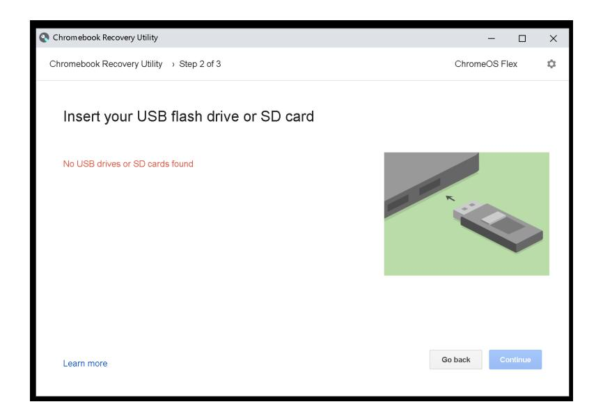
Insert a 8 Gigabyte or larger USB flash drive or USB SSD into a USB port of the computer. This USB device must have been previously formatted with the "FAT16" file format:
