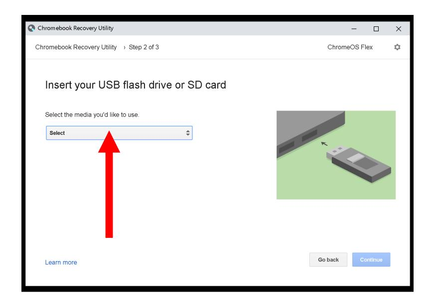
Use the left mouse button to click on name of the USB flash drive that you wish to make into a bootable installation media device for installing "Chromebook Flex" into ANOTHER computer:
